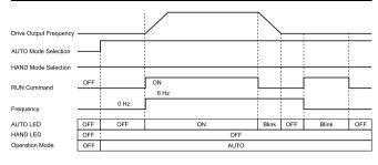
Figure 4.3 LEDs and Drive Operation in AUTO and HAND Modes
