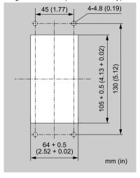
Figure 5.8 Panel Cut-Out Dimensions to Attach Inside Control Panel
