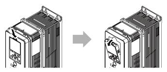
Figure 5.1 Remove the Keypad
