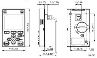
Figure 5.3 Exterior and Mounting Dimensions
