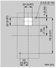
Figure 5.4 Panel Cut-Out Dimensions to Attach Outside of Control Panel
